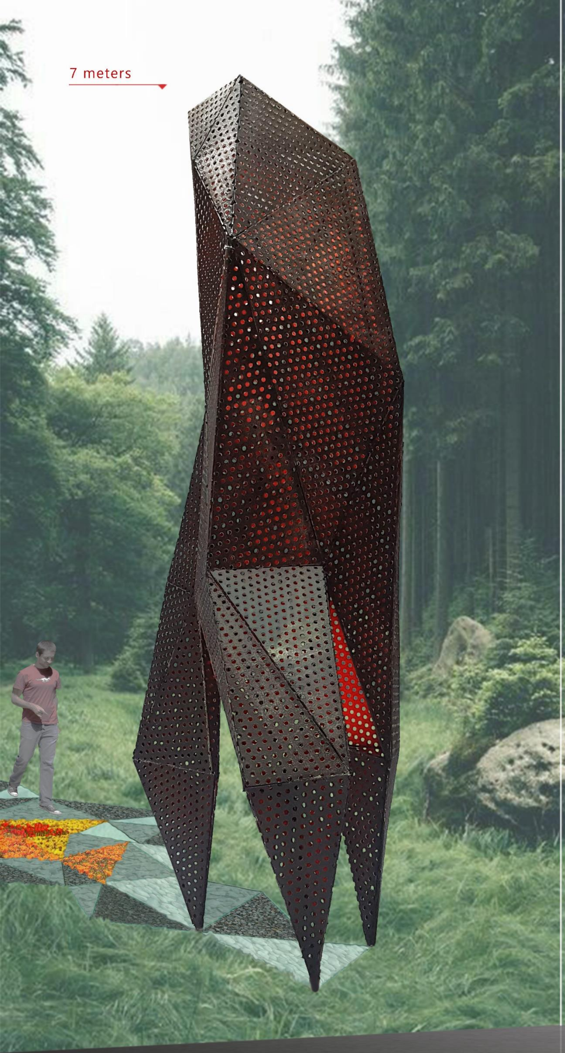
Construction - steel profile. Filling / walls - perforated plywood or metal plates- external side fired (black) oiled - inner side painted in red.
